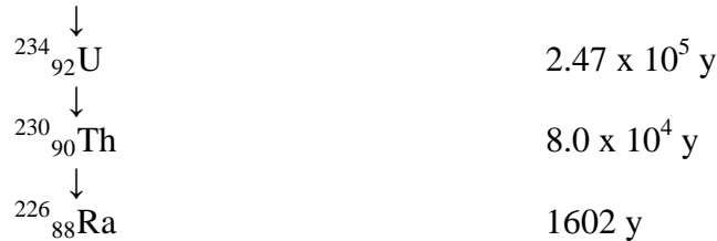
Chart 1: (Taken from [3].) This chart illustrates the decay scheme relationships between Uranium 238 and its daughter products down to Radium 226 together with the respective half-lives.
