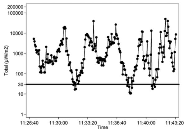
Figure 6. Total radiofrequency field exposure ( $\mu\text{W}/\text{m}^2$ ) of the lowest exposure round (151109, 10:50; mean exposure  $2,817.0 \mu\text{W}/\text{m}^2$ ) by walking across the station. The horizontal line represents the exposure limit of  $30 \mu\text{W}/\text{m}^2$  suggested by the BioInitiative Report (29).
