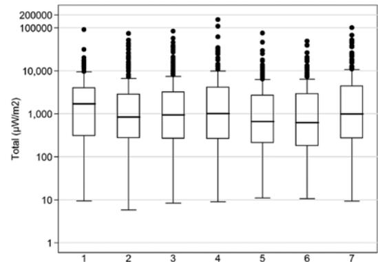
Figure 4. Box plot for total exposure in  $\mu\text{W}/\text{m}^2$  for the seven measurement rounds. The median is indicated by a black line inside each box; the bottom and top of the boxes show first and third quartiles; the end of the whiskers are calculated as  $1.5 \times \text{IQR}$  (interquartile range). Points represent outliers.
