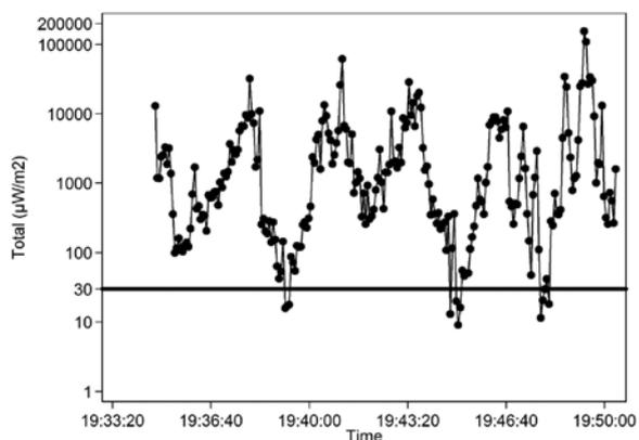
Figure 5. Total radiofrequency field exposure ( $\mu\text{W}/\text{m}^2$ ) of the highest exposure round (151108, 18:50; mean exposure  $4,891.2 \mu\text{W}/\text{m}^2$ ) by walking across the station. The horizontal line represents the exposure limit of  $30 \mu\text{W}/\text{m}^2$  suggested by the BioInitiative Report (29).
